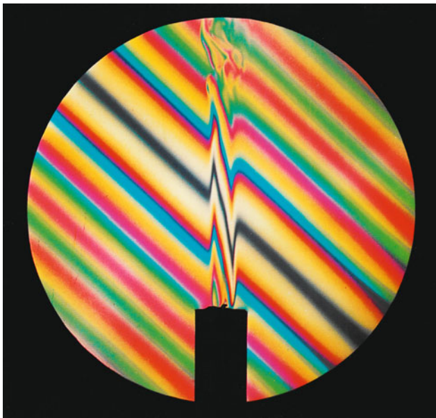
Fig. 8.46 Convection currents above a candle flame observed with a differential interferometer (interferometer with polarization) From: M. Cagnet, M. Francon, S- Malik: Atals optischer erscheinungen (Springer, Berlin, Heidelberg 1971)
