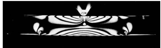
Fig. 8.54 Birefringence of a plexi glass rod induced by mechanical stress in the rod supported at two points and pressed in the midpoint
