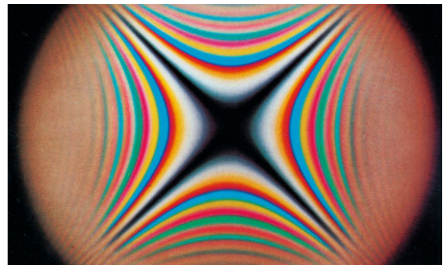
Fig. 8.55 Stress-induced birefringence detected in convergent light. Two equal quartz plates cut parallel to the optical axis are turned to a crossed position of their optical axes and are placed between two crossed polarizers. Convergent white light passes through the arrangement. From Francon et al. (1971)
