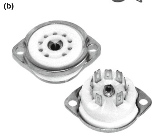
Fig. 5.57 a) Commercial pentode with tube socket, b) socket of an electron tube. Upper part: side towards the tube; lower part: side of the circuit
