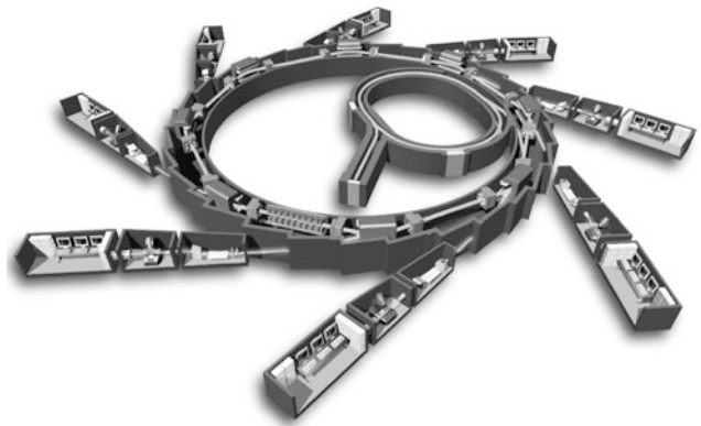
Fig. 6.36 Synchrotron SOLEIL in Gif-sur-Yvette near Paris with 8 beam lines and measuring stations The small ring in the inner part is the pre-accelerator for the electrons
